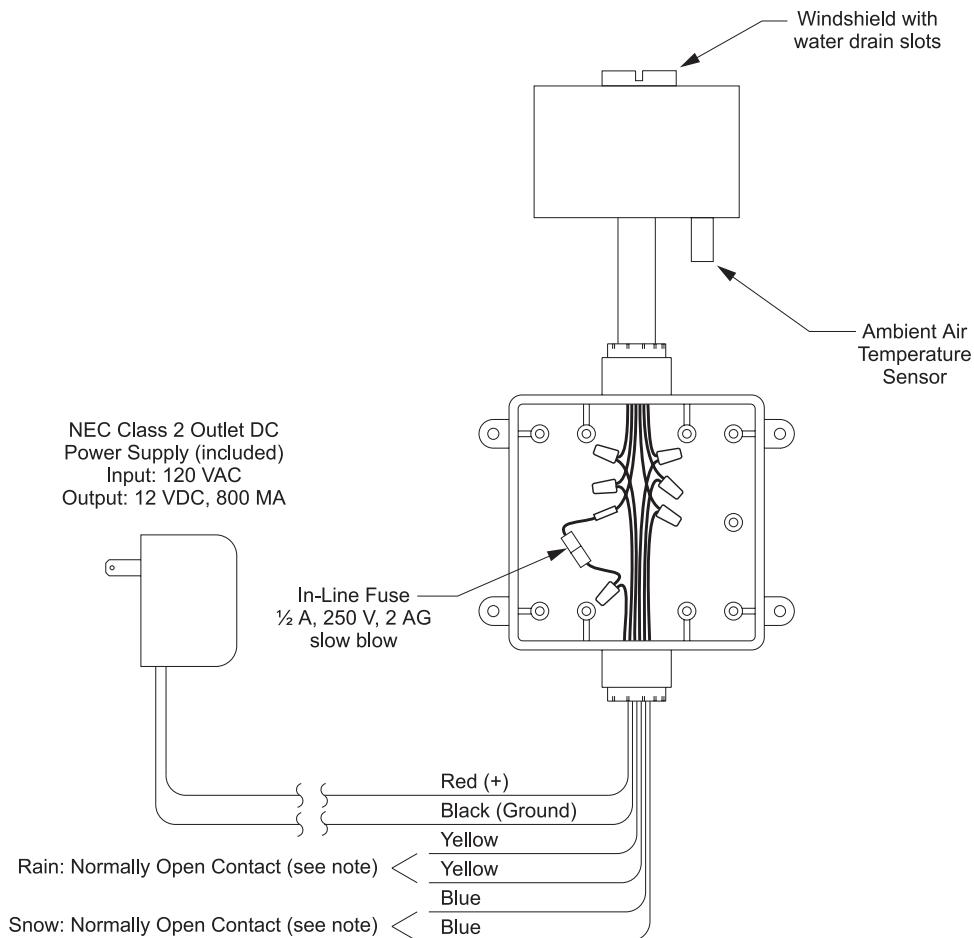
Note: Output relays have dry reed contact rated at 0.5 amps, 10 watts max
