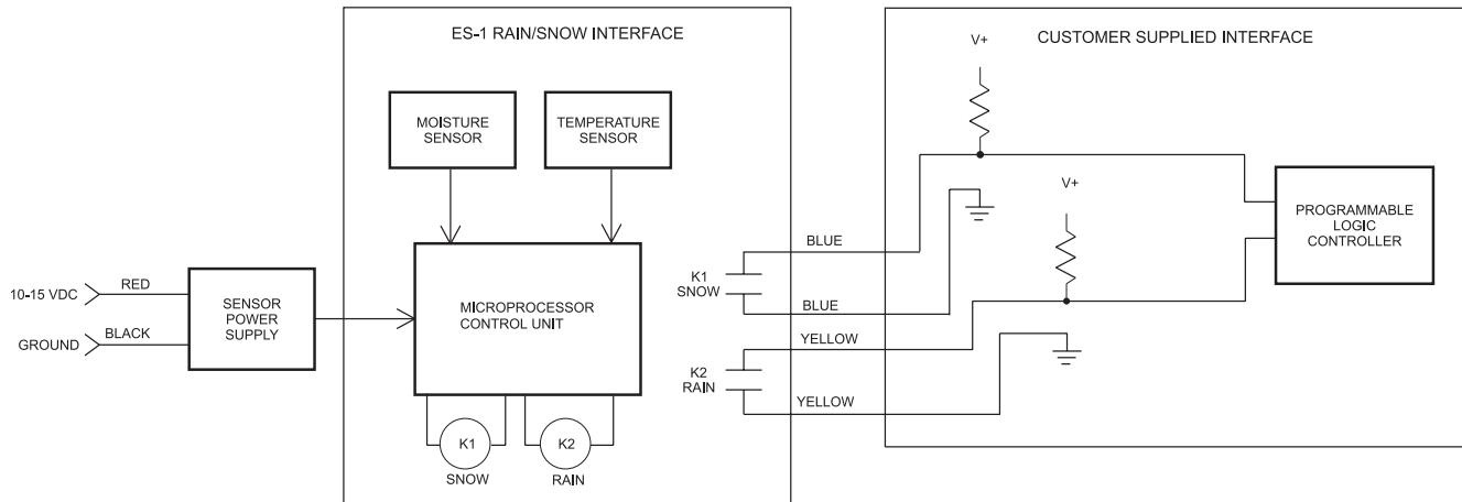
Figure 1. ES-1 Rain/Snow Interface block diagram.
