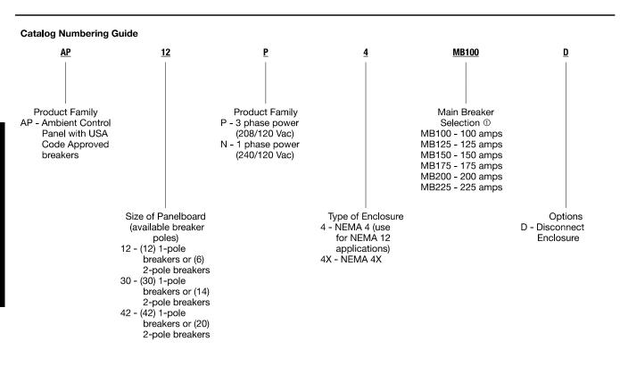
① Note: Standard 12-Pole option is limited to 100A maximum main breaker sizing.
